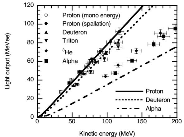
Fig. 7. Light output of BC501A liquid organic scintillator for proton, deuteron, triton,  $^3\text{He}$  nucleus and alpha particle. Marks indicate experimental results. Open circles are obtained by the mono-energy beam method, and other marks are by the spallation method. Lines indicate the formulas, solid and broken lines are proposed by Nakao[4] for proton and deuteron, chain line is by Cecil[5] for alpha particle
