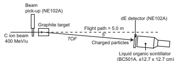
Fig. 1. Experimental arrangement of spallation method
