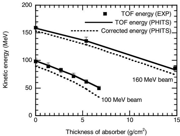
Fig. 6. Relationship between kinetic energy of incident beam and thickness of energy absorber. Marks are experimental data. Lines are calculated results by PHITS[6]. Broken lines were corrected the contribution of the energy loss at the Al case containing the liquid scintillation material
