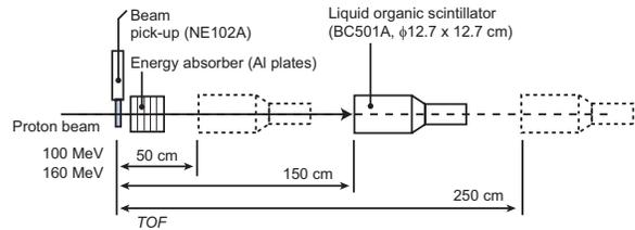
Fig. 4. Experimental arrangement of mono-energy beam method
