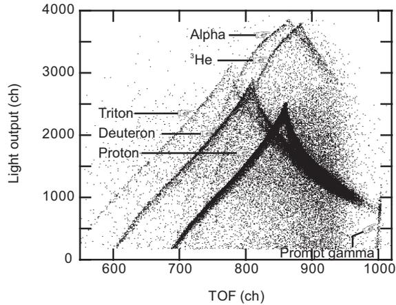
Fig. 2. Two-dimensional scatter plot of TOF and light output of liquid organic scintillator
