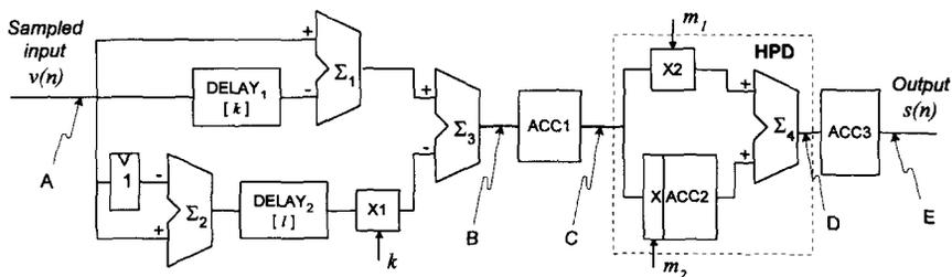
Fig. 6. Block diagram of the digital cusp-like shaper.
