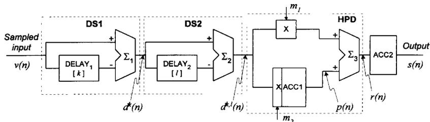
Fig. 4. Block diagram of the digital trapezoidal/triangular shaper. The elements are: DELAY<sub>n</sub> – a delay pipeline, Σ<sub>n</sub> – an adder/subtracter, ACC<sub>n</sub> – an accumulator, X<sub>n</sub> – a multiplier.
