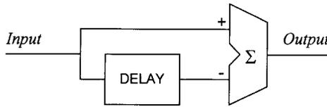
Fig. 1. Block diagram of the delay-subtract unit
