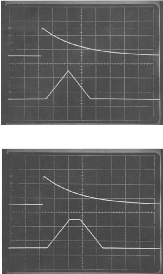
Fig. 5. Oscillograms of triangular and trapezoidal shapes at the output of a DAC connected to the digital pulse shaper. The upper trace in each of the oscillograms is the input exponential pulse. The time base is set to 2  $\mu$ s per division.
