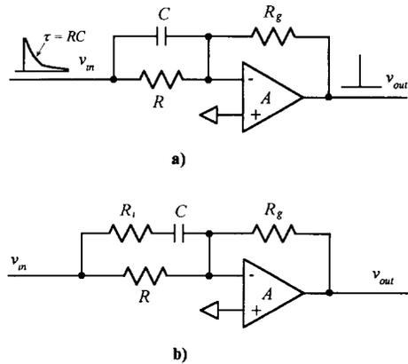
Fig. 3. Analog deconvolving circuits: (a) ideal and (b) practical ( $R_1C \ll RC$ ).
