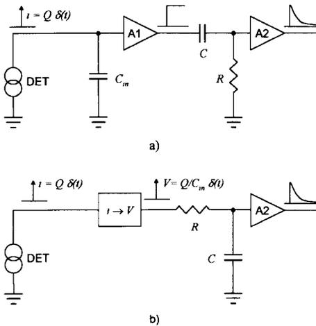
Fig. 1. Idealized detector–amplifier configuration.
