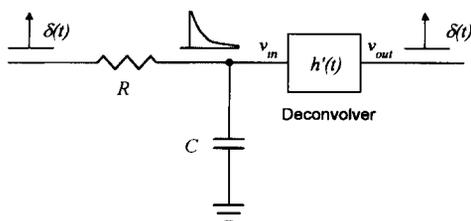
Fig. 2. Deconvolution of the signal from a low-pass network.
