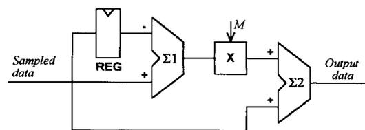
Fig. 5. Block diagram of the digital deconvolver. REG – one clock delay register,  $\Sigma 1$ ,  $\Sigma 2$  – arithmetic units, X – multiplier.
