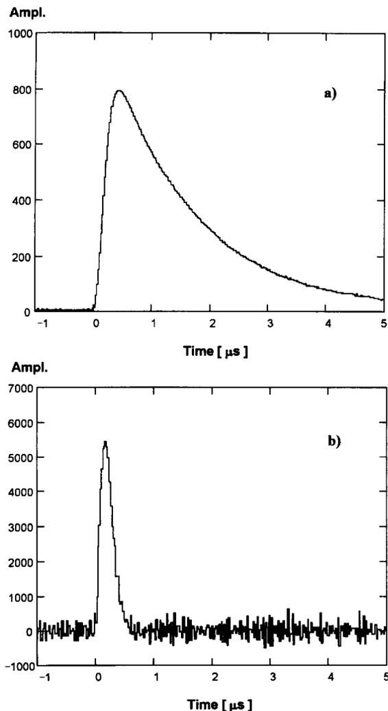
Fig. 6. Sampled exponential pulse (a) and digitally deconvolved signal (b).
