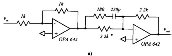
Fig. 4. Analog deconvolver (a) and oscillogram of the input and output signals (b). Trace 1 shows the input exponential pulse with decay time constant of 500 ns and trace 2 represents the deconvolver response.
