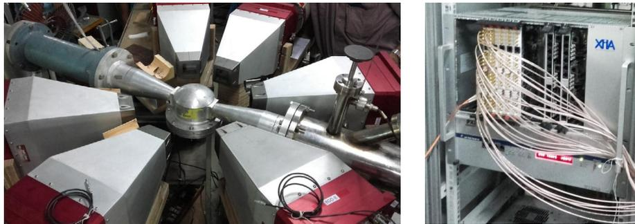
Fig. 2. (Colour online) The VENUS array [4] at the K130 cyclotron in VECC, Kolkata and the DAQ system based on Pixie-16 digitizer modules. The distance of the target position from the end cap of the detectors was 26 cm.
