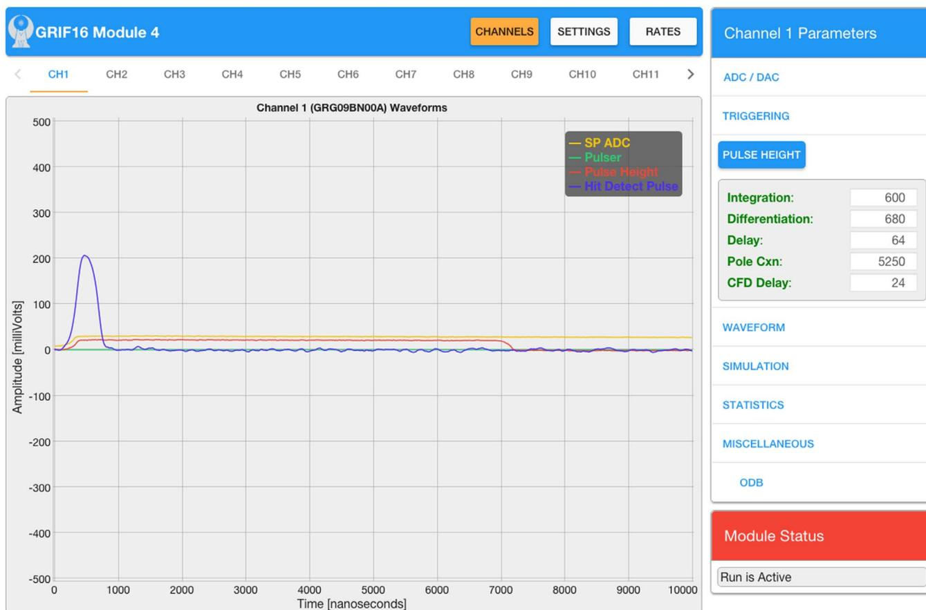
**Fig. 14.** Screenshot of an example GRIF-16 digitizer User Interface for a single channel. The waveforms update in real time similar to a digital oscilloscope. The menus on the right allow the user to change parameters of the signal processing algorithms.
