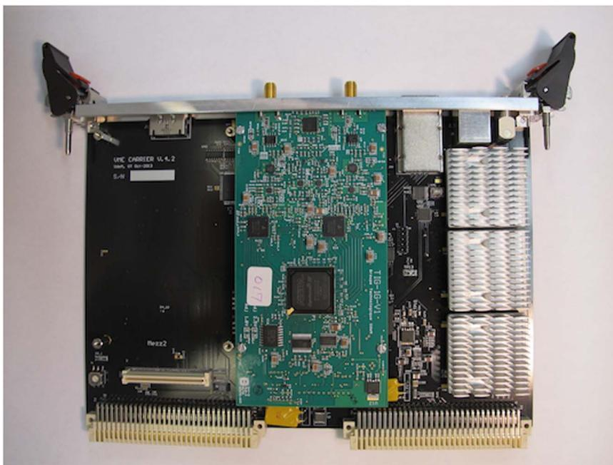
Fig. 3. Photograph of the GRIF-4G module. The lower mezzanine card is removed.
