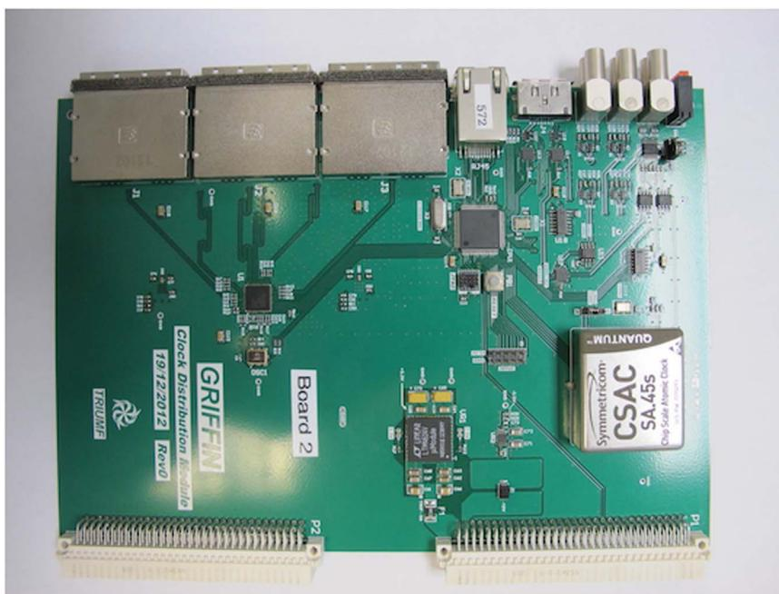
**Fig. 5.** Photograph of the GRIF-Clk Clock module. The Symmetricom Chip-Sized Atomic Clock can be seen at the lower right of the photograph.
