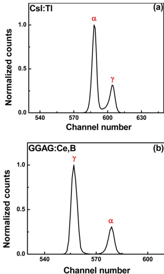
Fig. 7. PSD for alpha and gamma rays in (a) CsI:Tl and (b) GGAG:Ce,B crystals coupled to PMT from zero-crossing setup.
