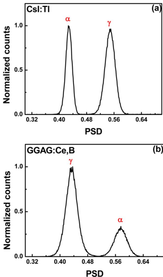
Fig. 8. PSD plots for alpha and gamma rays of (a) CsI:Tl and (b) GGAG:Ce,B crystals coupled to SiPM from Digitizer.
