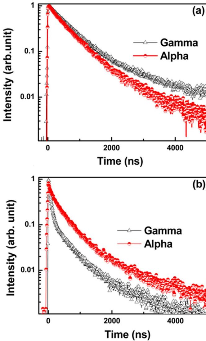
Fig. 4. Normalized scintillation decay curves measured with alpha and gamma sources for (a) CsI:Tl and (b) GGAG:Ce,B crystals coupled to PMT.
