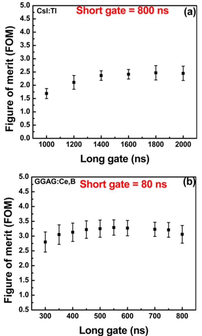
Fig. 5. The effect of long gate settings on figure of merit (FOM) measured for (a) CsI:Tl and (b) GGAG:Ce,B crystals coupled to PMT.
