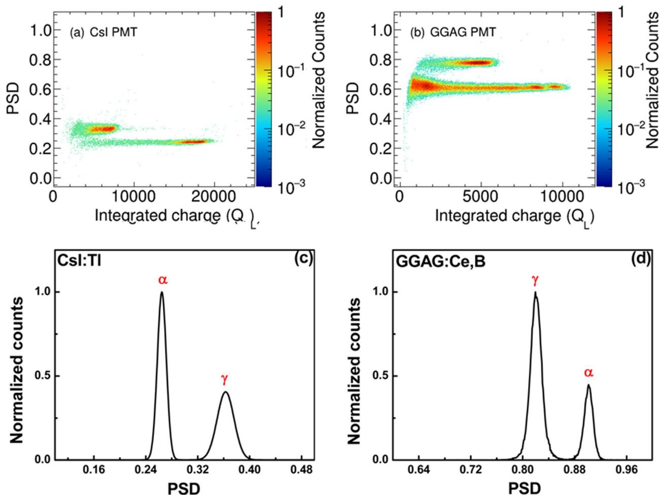
**Fig. 6.** Results of PSD measurement using digitizer for alpha and gamma rays of (a) CsI:Tl and (b) GGAG:Ce,B crystals coupled to PMT. The projection along X-axis is shown for (c) CsI:Tl and (d) GGAG:Ce, B.
