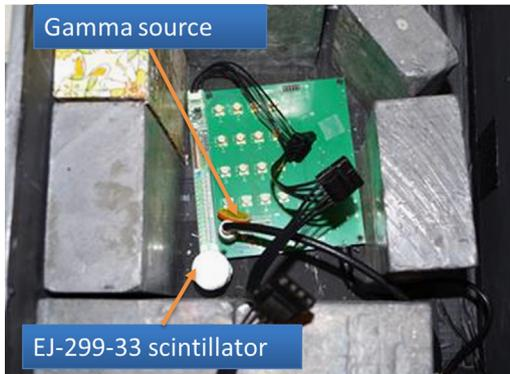
Fig. 4. The experimental setup for energy calibration.
