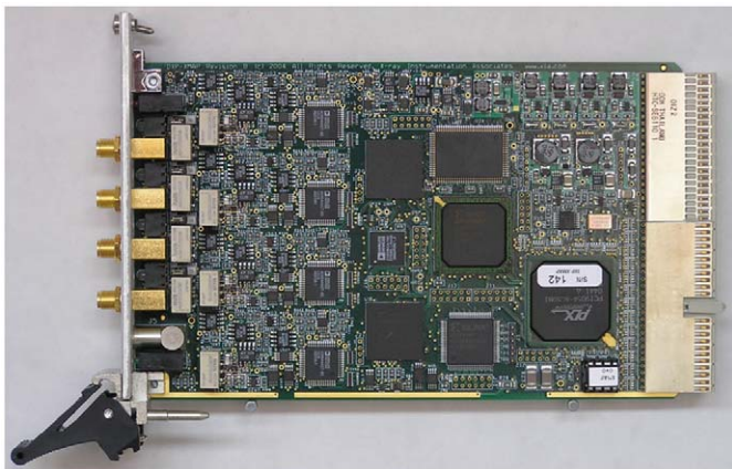
Fig. 9. xMAP high-speed digital X-ray spectrometer.
