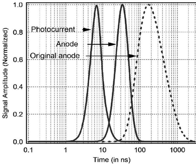
Fig. 1. Simulated anode signal shapes.
