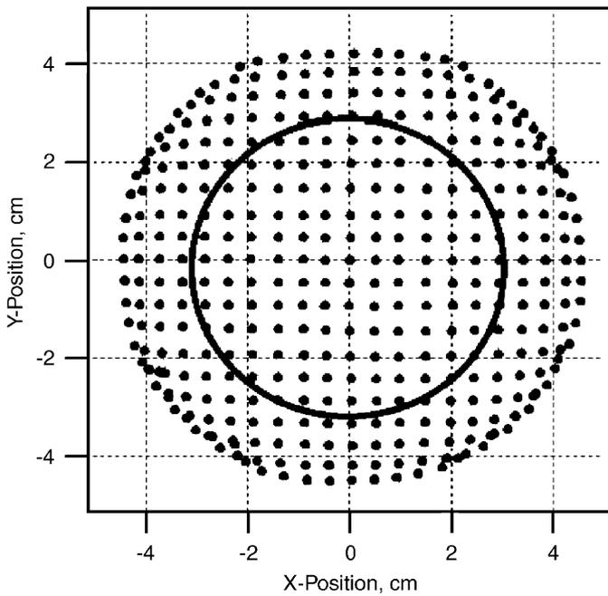
Fig. 5. R3292 Mapping function. Circle represents the active area (high linearity).
