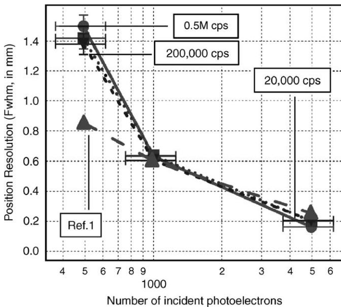
Fig. 6. Position resolution with number of incident photoelectrons and event rate (R2486). Ref. [1] refers to the position resolution reported from the device datasheet.
