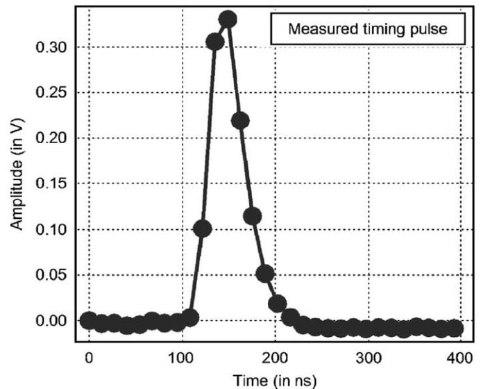
Fig. 4. Measured time signal (R2486). This signal was extracted by AC coupling the PSPMT dynode 12.
