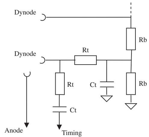
Fig. 3. Timing circuit.  $R_t = 50\ \Omega$ ,  $R_b = 200\ \text{k}\Omega$ ,  $C_t = 10\ \text{nF}$ .
