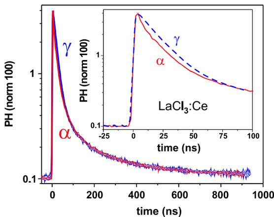
Fig. 1. Normalized light output from  $\text{LaCl}_3:\text{Ce}$  from  $\alpha$ -particles and  $\gamma$ -rays (dashed in inset figure). The pulse-height spectra are normalized to the same area.
