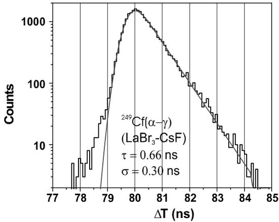
Fig. 2. Alpha-gamma time-to-amplitude spectrum and fit.
