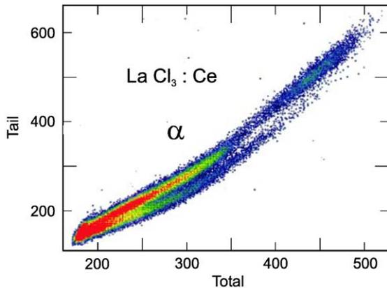
Fig. 3. Standard PSD plot of total (abscissa) and partial (ordinate) integration of the pulses produced by  $\text{LaCl}_3:\text{Ce}$  exposed to a  $^{232}\text{U}$  source. The locus for  $\alpha$ -particles shows two groups, one at lower energy composed of many closely spaced lines and a higher energy peak from the 8.8 MeV decay of  $^{212}\text{Po}$ . The  $e^-$  ridge is below that for  $\alpha$ -particles.
