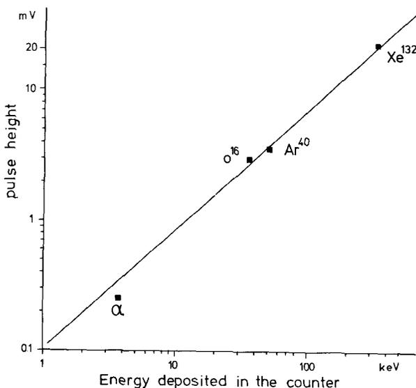
Fig. 3. Pulse height vs energy deposited in a PPAC with a 1 mm gap. The counter was operated in 10 torr i-butylene. The applied voltage was 490 V.
