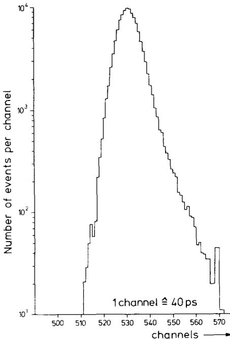
Fig. 6. Coincidence curve (measured with  $\alpha$ 's) of two PPACs with  $0.8 \text{ cm}^2$  and  $50 \text{ cm}^2$  surface and a gap of 1 mm.
