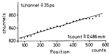
Fig. 5. Shift of the timing signal as a function of the impact point of the particle on the PPAC ( $2 \times 25 \text{ cm}^2$  surface, gap 1 mm).
