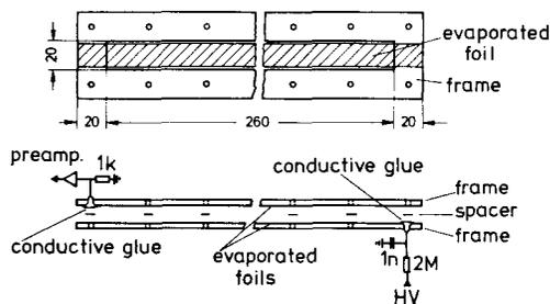
Fig. 1. Schematic view of a parallel plate avalanche counter.
