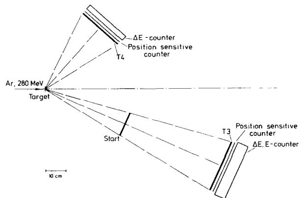
Fig. 7. Scheme of the experimental set-up to measure the deep inelastic process  $\text{Ar} \rightarrow \text{Ni}$ . The counters labelled START, T3 and T4 are parallel plate avalanche counters.
