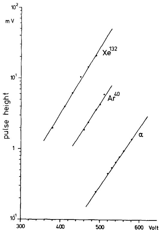
Fig. 4. Pulse height vs applied voltage for different particles. The gap was 1 mm, the counting gas was i-butylene at 10 torr.
