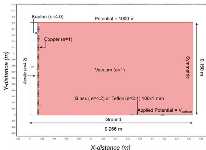
Fig. 10. Electrostatic model of the XIA UltraLo-1800.
