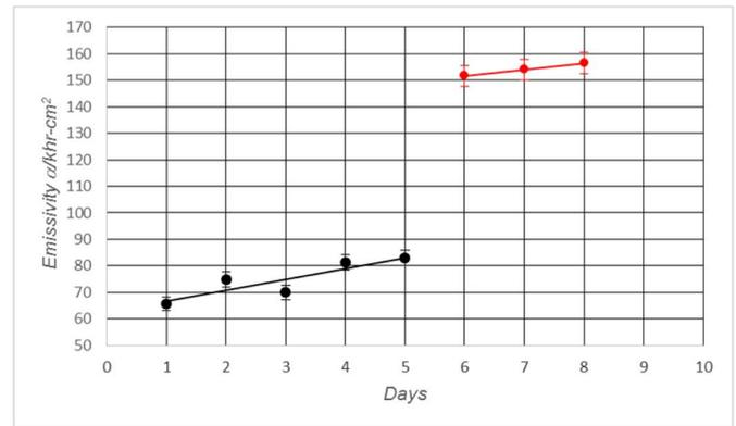
Fig. 8. The alpha particle emissivity of the charged glass measured for 5 days, then for 3 days after a piezoelectric antistatic tool was used to discharge the sample.
