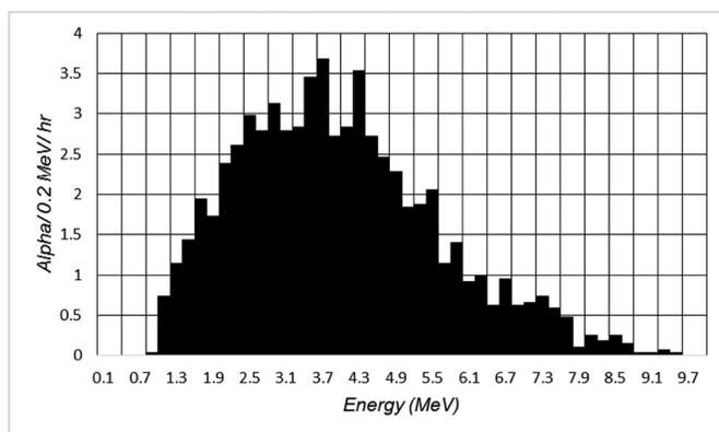
Fig. 4. Energy spectrum of the uncharged 446 cm<sup>2</sup> glass sample.
