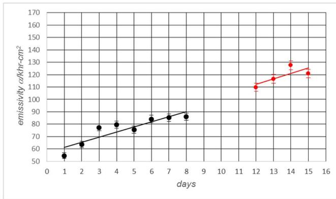
Fig. 6. The alpha particle emissivity of the charged glass measured for 8 days, then for 4 days after a 3 day period where the  $^{230}\text{Th}$  source was left in the counter (with the high voltage off) to dissipate the static charge.
