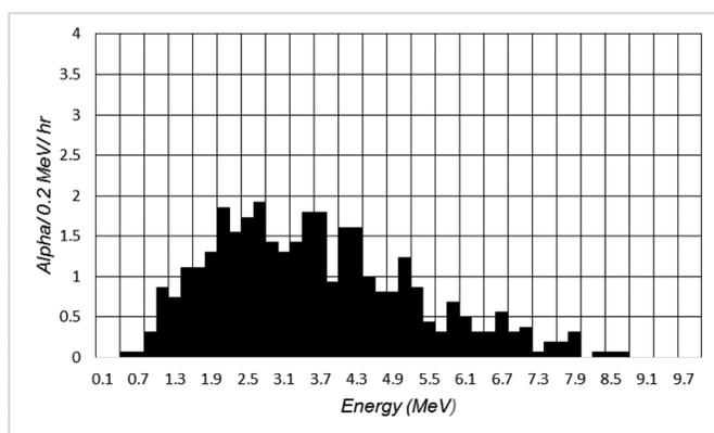
Fig. 5. Energy spectrum of the charged 446 cm<sup>2</sup> glass sample.
