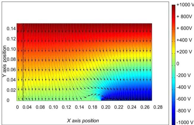
Fig. 12. The results of an electrostatic model of the XIA UltraLo-1800 ionization counter with a 200 mm  $\times$  200 mm Teflon sample charged to  $-1$  kV.
