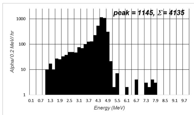
Fig. 3. Energy spectra of  $^{230}\text{Th}$  source placed on the charged glass.
