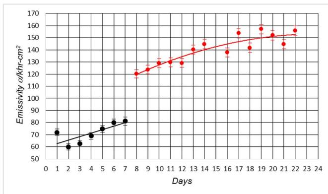
Fig. 7. The alpha particle emissivity of the charged glass measured for 7 days, then for 14 days after a  $\sim 0.1 \mu\text{Ci } ^{241}\text{Am}$  source was placed in 9 locations in a  $3 \times 3$  pattern for 5 minutes each.
