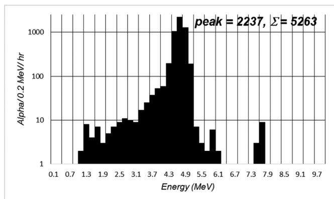
Fig. 2. Energy spectra of  $^{230}\text{Th}$  source placed on the tray liner.
