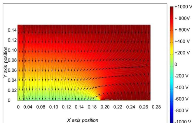
Fig. 11. The results of an electrostatic model of the XIA UltraLo-1800 ionization counter with a  $200 \text{ mm} \times 200 \text{ mm}$  glass sample charged to +1 kV.
