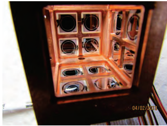
Fig 4. Inside view of the partially constructed detector cuboid, showing three window frames glued in place and the gas inlet hole, (visible near the center of the picture).
