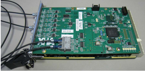
Fig. 1. Picture showing a MicroCAL-T128 board consisting of a TDM daughter board and a main board.
