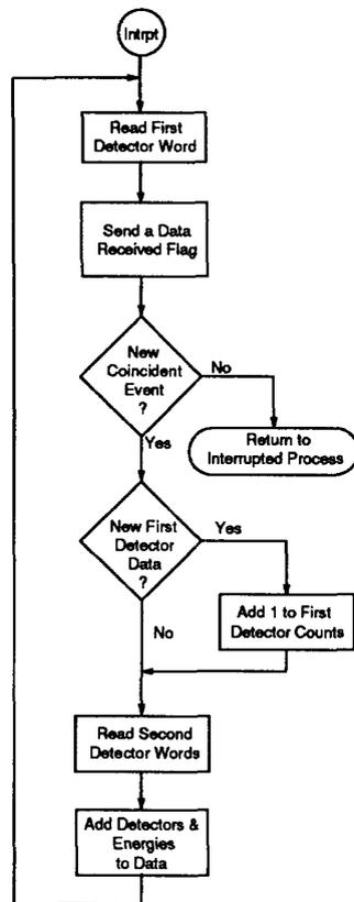
Fig. 4 Interrupt routine flowchart.
