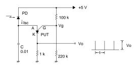
$\begin{array}{l} \text{PD} \hspace{0.1cm}:\hspace{0.1cm} \text{S2386-5K} \\ \text{PUT:} \hspace{0.1cm} \text{N13T2} \hspace{0.1cm} (\text{NEC}), \hspace{0.1cm} \text{TN41B} \hspace{0.1cm} (\text{TOSHIBA}), \hspace{0.1cm} \text{etc.} \\ \text{f} = \frac{1}{t} = \frac{1}{\sqrt{u}} \times \frac{\text{lsc}}{C} \hspace{0.1cm} [\text{Hz}] \end{array}$
