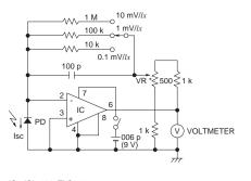
IC : ICL7611, TLC271, PD: S7686 (0.45 µA/100 lx) ' Meter calibration trimmer potentiometer
