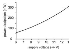
The power dissipation of the CR-112 is shown to the left as a function of supply voltage. The minimum supply voltage for good operation is  $\pm 6\text{V}$ . Any supply voltage applied in excess of this figure does not change or improve CR-112 performance, but instead results in unnecessary power dissipation.
