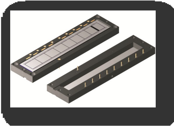
The MSPAD 1x9(SS) in a single assembly configuration or two silicon devices mounted back-to-back in a single package.
