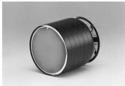
Figure 9-26: Grid type dynode photomultiplier tube
