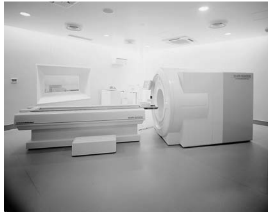
Figure 14-9: External view of a whole-body PET scanner (Hamamatsu Photonics SHR-92000)
