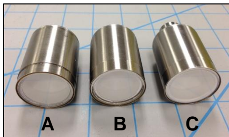
Ruggedized hermetic package sapphire window
