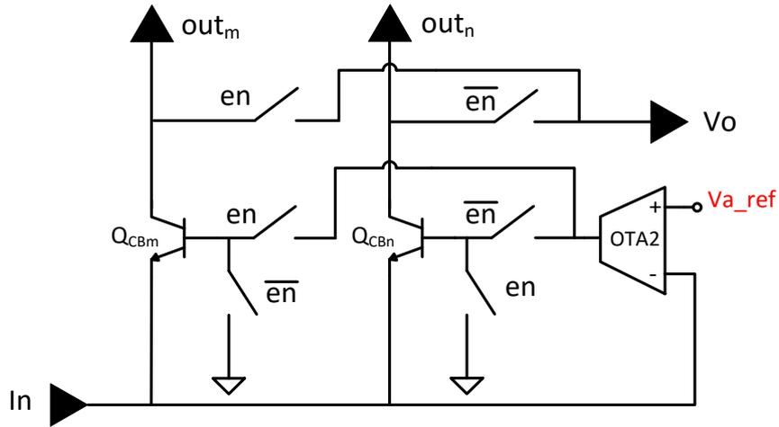
Figure 2: Implementation of the summing current switch.
