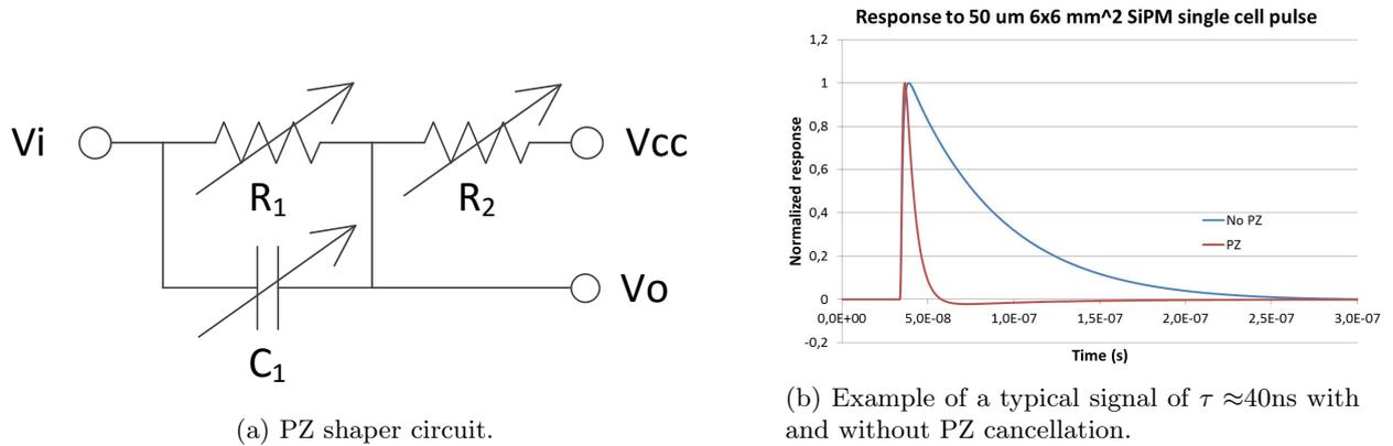
Figure 3: Pole-zero compensation.
