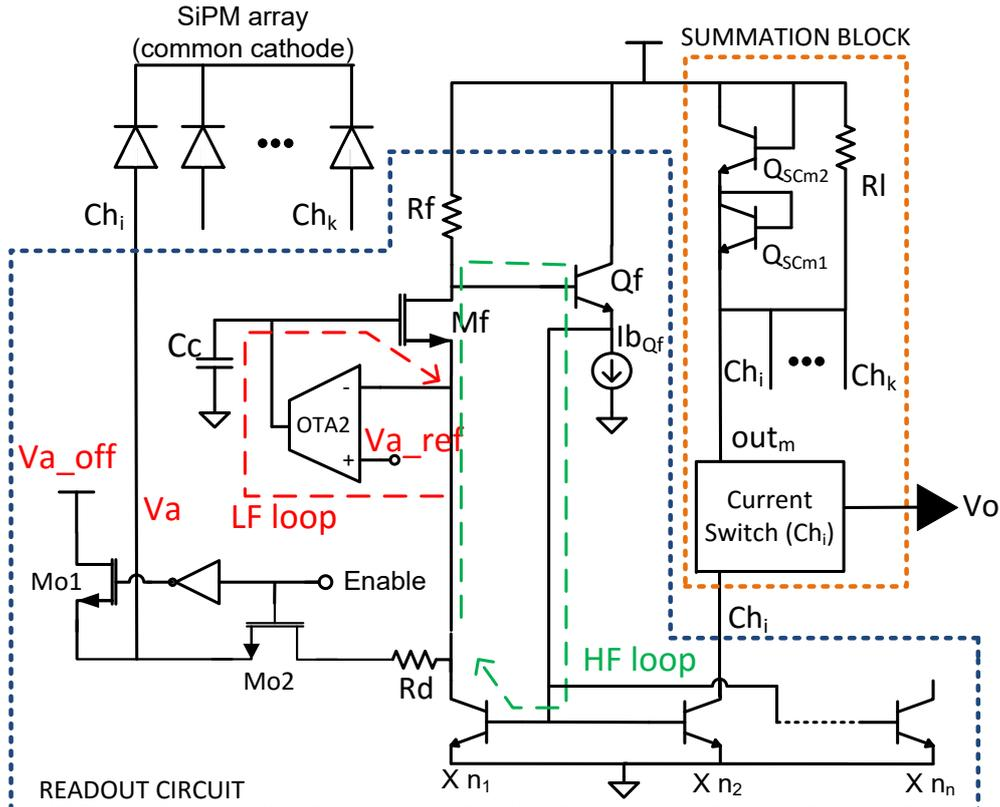
Figure 1: Input current stage including the readout circuit and the summation block.
