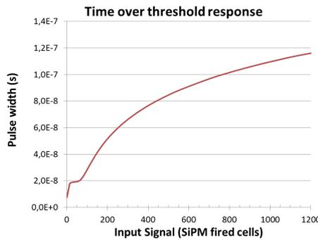
Figure 7: Time over threshold response for different input fired signals.
