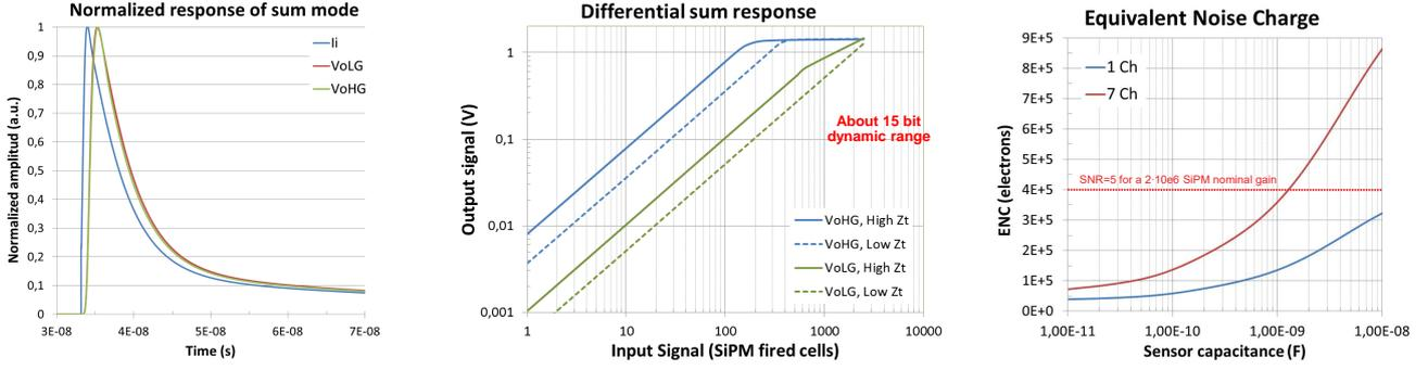
(a) Transient simulation of the normalized input and output response.
