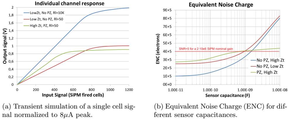
Figure 6: Analog single channel characteristics.
