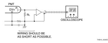
Figure 5-36: Waveform observation using an oscilloscope
