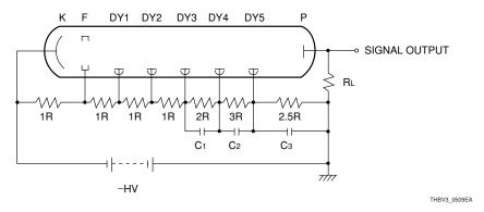
Figure 5-9: Pulse output linearity countermeasures using decoupling capacitors and tapered voltage-divider circuit
