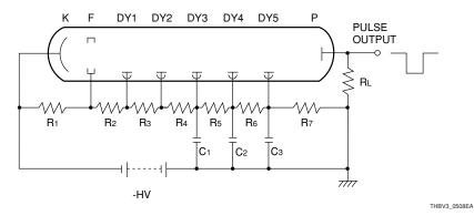
Figure 5-8 (2): Voltage-divider circuit with parallel-connected decoupling capacitors
