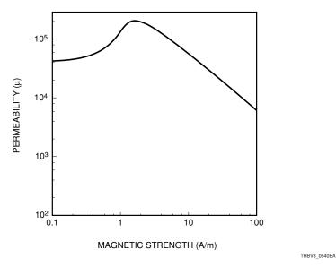
Figure 5-40: Permeability and external magnetic field
