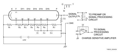
Figure 5-24: Cathode grounding scheme in pulse operation
