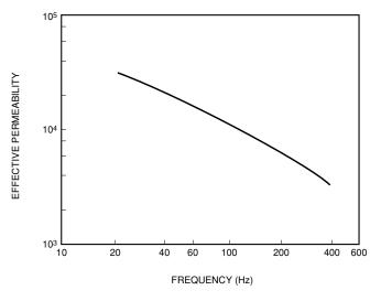
Figure 5-42: Frequency characteristics of a magnetic shield case
