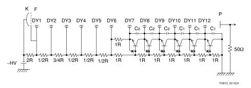
Figure 5-15: Voltage-divider circuit using transistors
