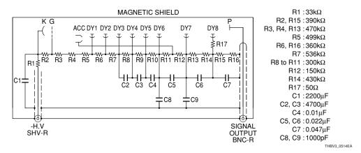
Figure 5-13: Fast-response voltage-divider circuits
