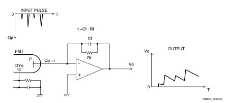
Figure 5-33: Pulse input type charge-sensitive amplifier
