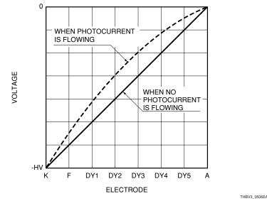
anode voltage is kept constant by the high-voltage power supply, the loss of the interstage voltage at the latter stages is redistributed to the previous stages so that there will be an increase in the interstage voltage.
