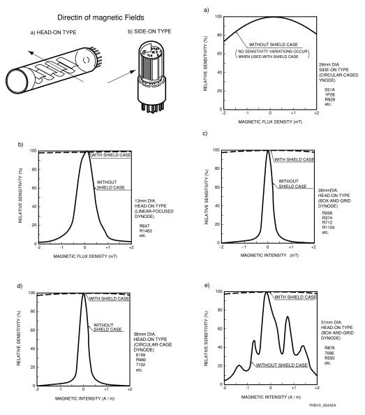
Figure 5-44: Effect of magnetic shield case
