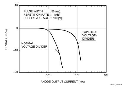
Figure 5-10: Linearity characteristic using a tapered and a normal voltage-divider circuit
