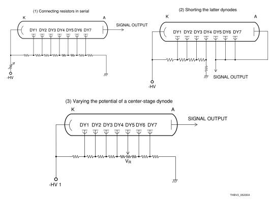
Figure 5-20: Anode sensitivity adjustment circuits
