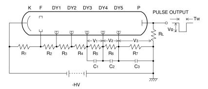
Figure 5-8 (1): Divider circuit with serial-connected decoupling capacitors
