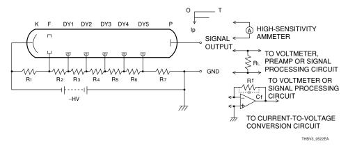
Figure 5-22: Anode grounding scheme in DC operation
