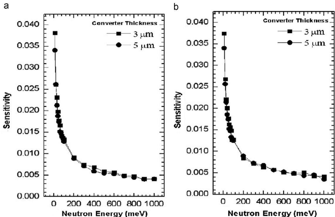
Fig. 3. Detection response evaluated for the double-layer GEM with 3  $\mu\text{m}$  and 5  $\mu\text{m}$  converters, as a function of thermal neutron energies. (a) QGSP\_BIC\_HP, and (b) QGSP\_BERT\_HP.
