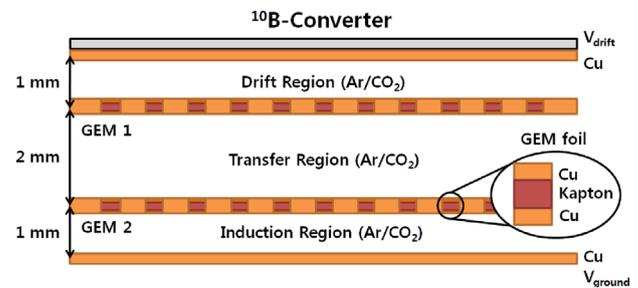
Fig. 1. A schematic view of the converter-based GEM detector.
