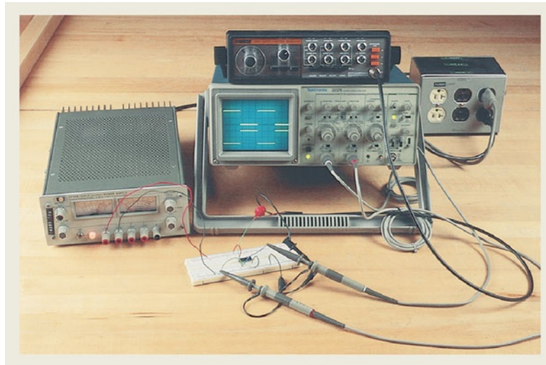
Figure 3–28 Timing analysis of an inverter gate: (a) waveform sketch and (b) oscilloscope display.
