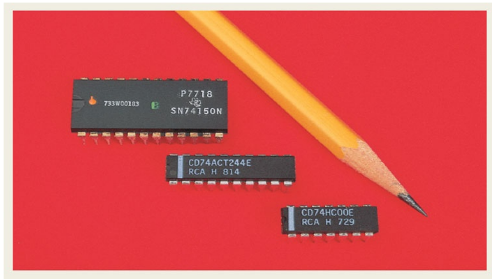
Figure 2-40 Photograph of three commonly used ICs: the 74HC00, 74ACT244, and 74150.
