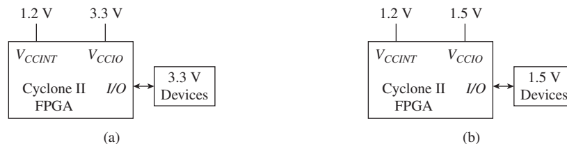
Figure 9–35 Interfacing an FPGA to different I/O devices: (a) the 3.3 V V_{CCIO} I/O configuration; (b) the 1.5 V V_{CCIO} I/O configuration.
