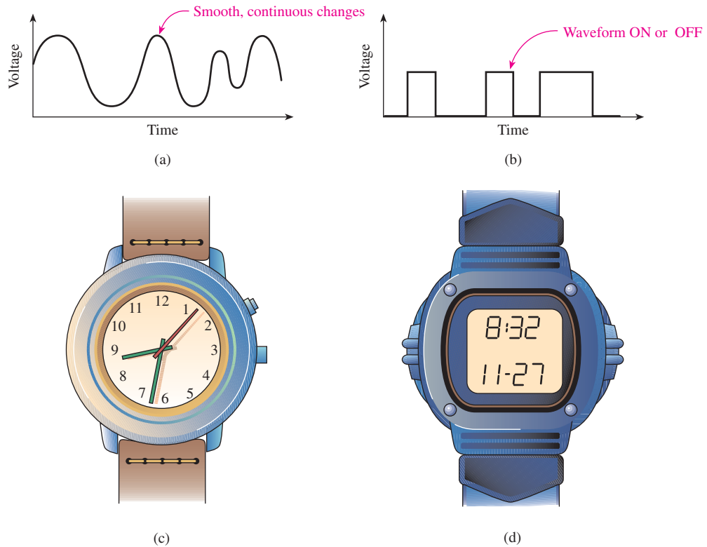
Figure 1-1 Analog versus digital: (a) analog waveform; (b) digital waveform; (c) analog watch; (d) digital watch.
