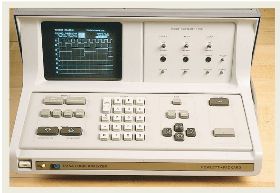
Figure 12–12 MOD-16 ripple counter: (a) Block diagram; (b) waveforms; (c) counter displayed on a logic analyzer.
