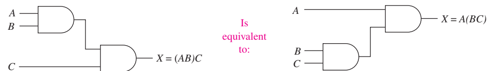
Figure 5-11 Using the associative law of multiplication to rearrange the grouping of AND gates.
