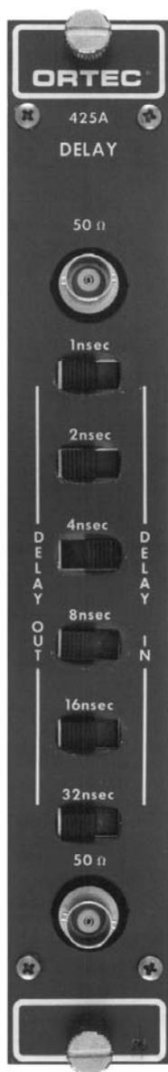
The ORTEC Model 425A Nanosecond Delay provides a calibrated delay for any type of signal in 1-ns steps from 0 to 63 ns. Longer delays can be obtained by cascading several Model 425As. The delays are accomplished with RG-58A/U coaxial cables that are interconnected by stripline sections. No power is required to operate the instrument.
