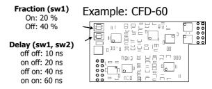
For other CFD delays see section "Types and ordering" See also label inside the movable module side plate.
