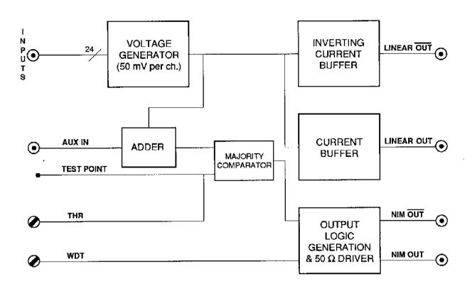
Figure 1 - Functional Block Diagram of the N 408 Module
