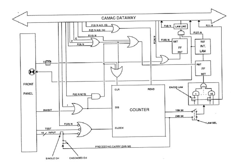
Figure 2 Functional Block Diagram of the Module.
