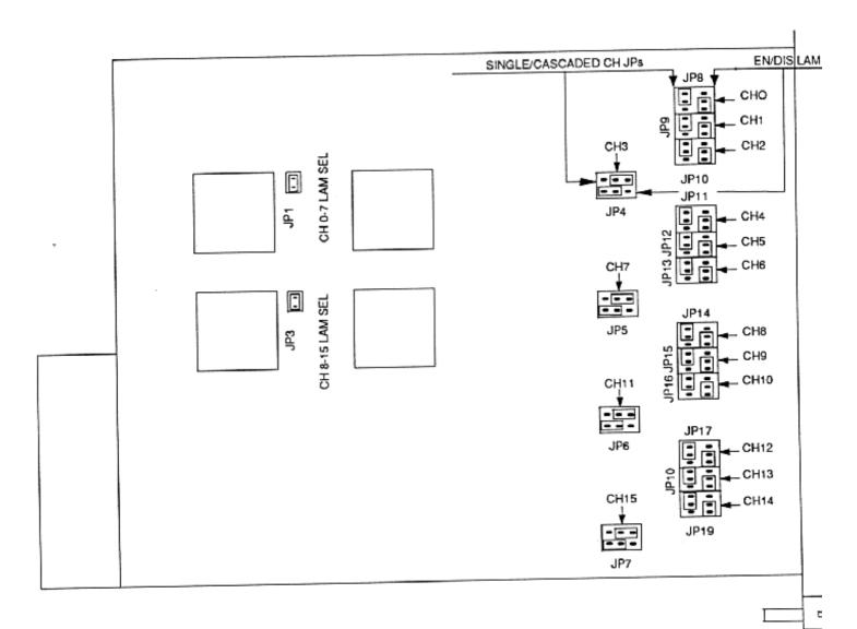
The module comes from CAEN with the internal jumpers configured as shown in figure above.
